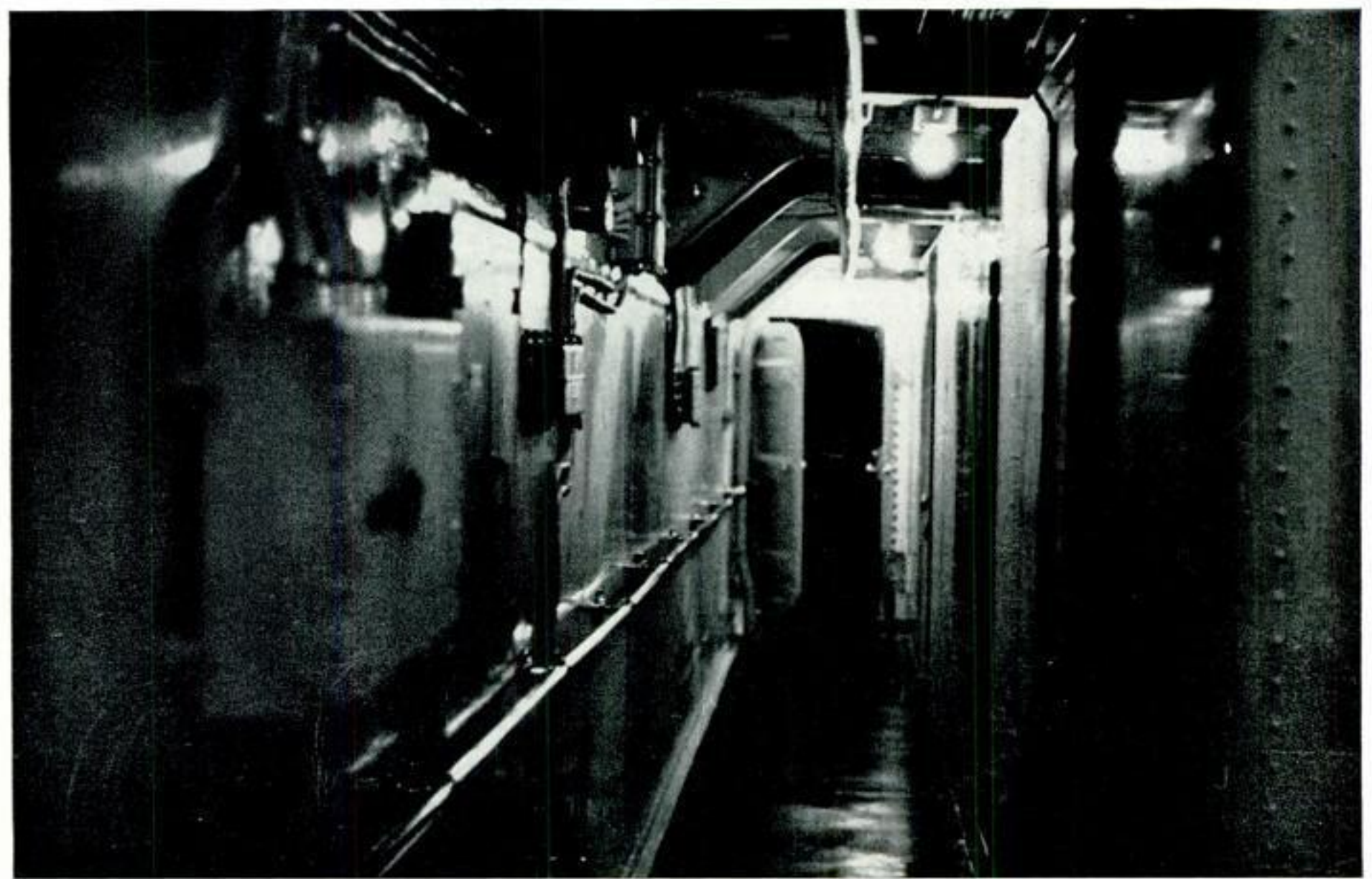
Handrails are screwed into the walls of the corridor leading to the President's quarters. At one end of this corridor is a door from which the high sill has been removed. At the other end is the private elevator.
