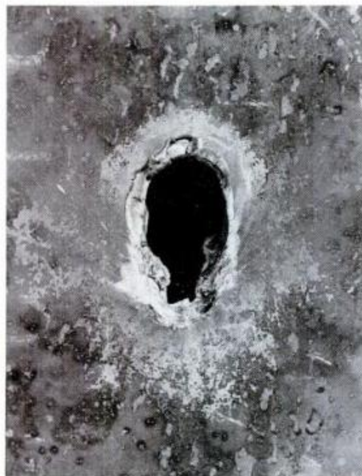
PUNCTURED STEEL has this gaping hole after 37-mm shell tears through it. Plate is \frac{3}{4} -inch thick.
