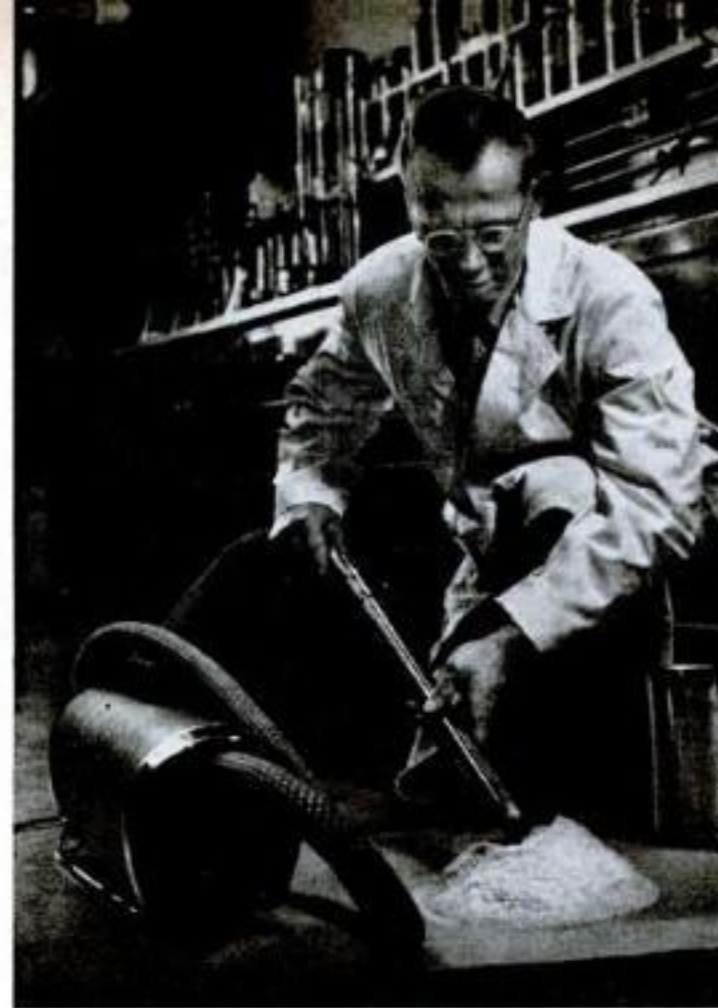
VACUUM CLEANER tests detergent to see if it will be affected when blown through factory pipes.
