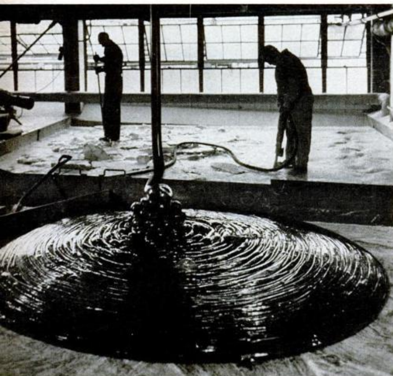
FALLING PLASTIC pours from overhead kettles onto floor of Springfield, Mass. plant. Power hammers break it up for packaging after it has hardened.
