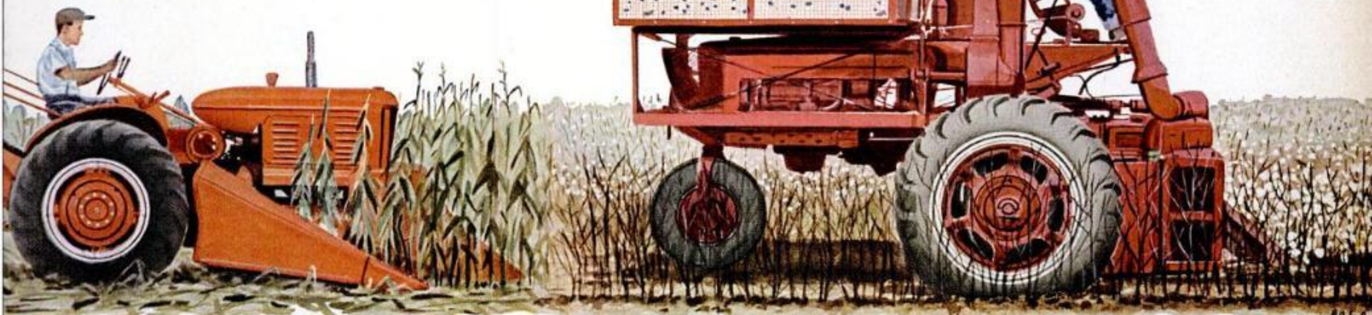
CORN PICKER , made by Allis-Chalmers for $840, is a shell which fits over a regular tractor. Ears are snapped from stalks, husked and dropped from feeder (left). Present pickers are used on feed corn only, but new machines are being developed for sweet corn.
